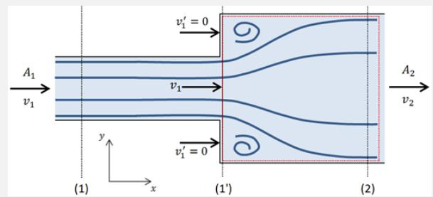
The continuity equation (eq 12, 13, 14) can be applied for the pipe expansion.
