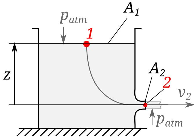
Setting the reference point at the top of the tank, we have  $z_1 = 0$  and  $z_2 = z$ , which brings the velocity at the top of the tank to be zero, so  $\frac{v_1^2}{2} = 0$ . Since  $p_1 = p_2 = p_{atm}$ , the specific form of Bernoulli can be simplified to:
