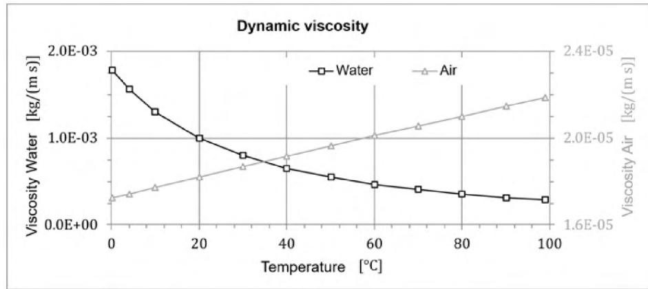
Viscosity of a liquid fluid **decreases** with increasing temperature, while viscosity of a gaseous fluid **increases** with increasing temperature.
