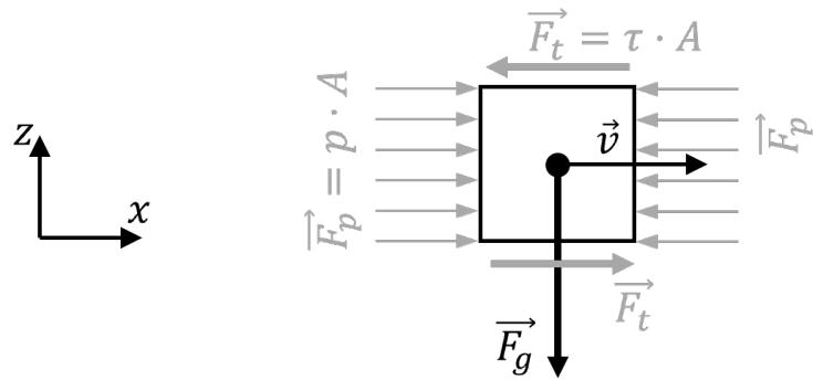
Surface forces act on the interfaces of a fluid body and are introduced by direct contact of the environment. Fluids also cause surface forces on their surroundings.
